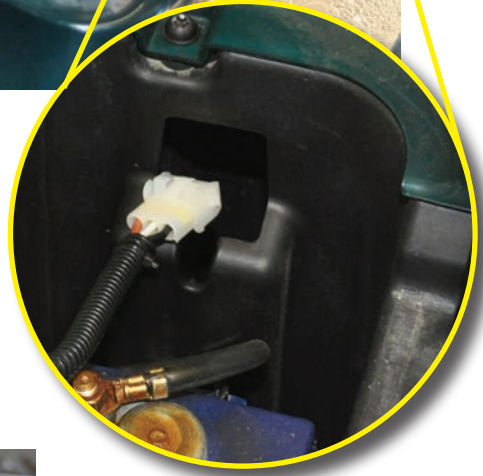
Feed through hole in tail light position on each side of vehicle
