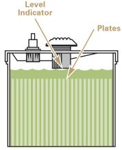
Maintain electrolyte level from at least 1/2-inch (13 mm) above plates to 1/4-inch (6 mm) below level indicator
