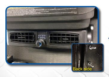
Attach fan to floor using four 6mm x 45mm hex head bolts as shown. Use rubber side of washer at fan bracket and underneath cart to seal hole. Once all 4 bolts are in place, tighten hardware. Route harness under cart to battery compartment and secure to frame using supplied zip ties. See STEP 9 for In-Line fuse instructions.
