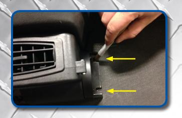
Find desired location as high up floor board as possible. Mark locations of bolt holes with a marking pen.
