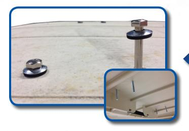
Insert the four 6mm x 45mm bolts through the top of the roof with rubber side of washer down as shown. If you are installing the fan on a TXT the four 6mm x 70mm bolts are needed.
