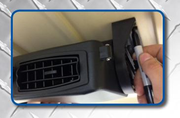
With the help of an assistant mark the desired location you want to mount the fan. Use a tape measure to square the brackets to ensure proper alignment.
