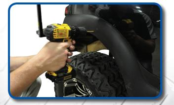
Drill first hole using a 9/32" drill bit. Ensure area behind body work is clear to avoid potential damage to wiring or other bodywork. Insert barbed push rivet half-way to secure fender flare. Check other marked holes to ensure proper placement before drilling. Once sure of placement, rotate fender flare out of the way and drill other holes.
