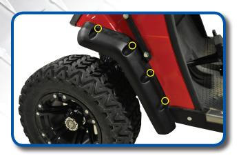
Push the first rivet in to secure fender flare and then insert other rivets.
