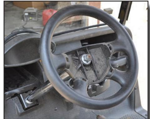
Loosen and remove nut from steering column spindle.
