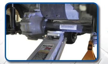
Place jack under rear end as shown. The jack is required to lower the rear end to complete the following steps.
