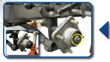
Remove dust cap, cotter pin, spindle nut and wheel hub. Retain hub and hardware.
