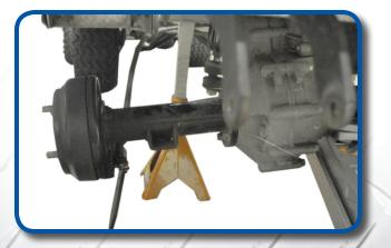
Use the jack to lower the rear end. Reposition spring above the axle and remount to factory mounting points using retained hardware from Steps 20 and 21. Attach bolt from hardware pack through the factory lower bracket. This bolt does not serve as a fastener, its only purpose to provide the proper placement of the bracket in the axle. Tighten all hardware.
