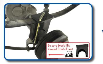
Place the rear shock mounting plate on top of leaf spring. Insert the lift block between the leaf spring and axle and then insert the provided U-bolt through top of the rear shock mounting plate. Attach shock to rear shock mounting plate.
