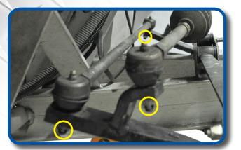
Remove cotter pins and castle nuts from steering linkage and drag link. Retain Hardware.
