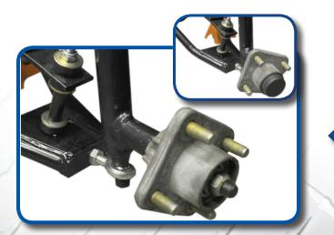
Reattach hub and dust cap using hardware retained from Step 4.
