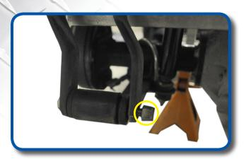
Remove rear hardware from leaf spring and retain. \*Check spring bushing for rust and wear. Replace if necessary.
