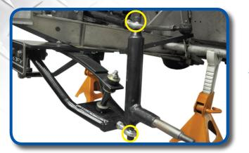
Attach spindles on both sides using hardware provided and tighten. DO NOT use thread locking adhesive until the end of installation. This will help with aligning of front tires.
