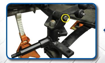
Remove A-Arm bolt from factory spindle on both sides. Do not retain bolts.
