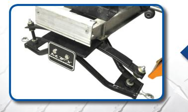
Attach the Main Suspension Assembly using hardware retained from Step 9 and tighten. \*A floor jack is recommended to help hold suspension assembly in place while you get the bolts started. A) Attach A-arm to shock using 8x50mm supplied hardware.B) Attach a-arm to bracket using 8x120mm supplied hardware and tighten.
