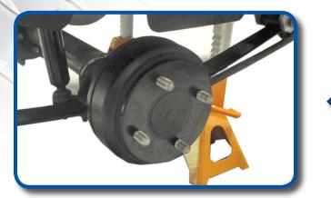
Chock front wheels. Lift up the rear of the cart using a jack. Use jack stands on the frame of the cart on each side to hold it up. Remove rear wheels using 19mm socket.
