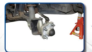
Use 19mm socket remove front wheels and then remove dust cover, cotter pin, and hub. Retain hardware. Using a 17mm socket and 11/16 wrench. Disconnect steering linkage by removing cotter pin and castle nut. Separate ball joint from spindle. Retain hardware.
