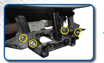
Using 14mm wrench and socket. Remove bolts from control arm assemblies. Retain hardware.
