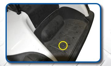
Use 10mm socket to remove bolt from bagwell. Drill 7/16 hole through the bagwell in the location shown.
