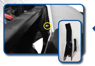
Using 14mm socket and wrench to attach Rear Mounting Bracket with retained hardware from step 15.
