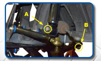
A) Using 14mm socket and wrench attach supplied shock to upper A-arm.B) Attach steering linkage to new spindle as shown. Using 14mm socket and wrench attach new shock to cart shock mount using retained hardware from step 5.
