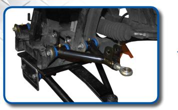
Attach upper A-arms using the 14mm socket and hardware retained from Step 5.
