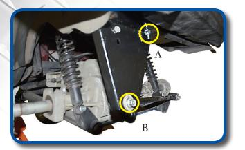
(A) Using supplied 10x90mm bolt. Insert through 7/16 hole drilled in bagwell and secure new sway bar bracket.(B) Attach sway bar to new bracket as shown using retained hardware using 17mm socket and wrench tighten all hardware.
