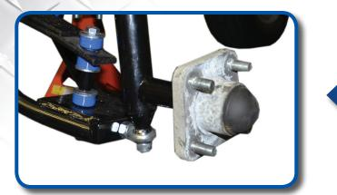
Attach hub and dust cover using retained hardware. Install wheels and re-attach bumper.
