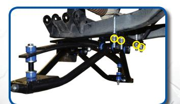
To attach main suspension assembly, install supplied U-Bolt on rear of assembly. Do not tighten.
