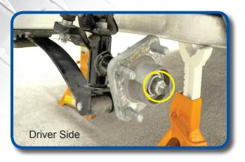
Using a 21mm Socket remove and retain hub and flange nut. Repeat on passenger side.
