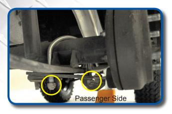
Using a 5/8" Socket loosen the U-Bolts on the passenger side.
