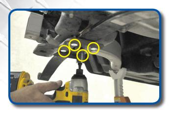
Using a 1/2" Socket remove spring plate and leaf spring. Retain spring plate, discard hardware and spring.
