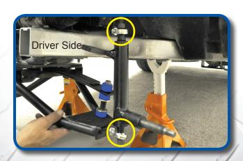
Note: Before attaching spindles, adjust heim joints so there is approximatly 1/4" of thread showing.
