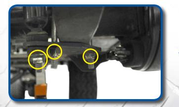
Loosen the factory passenger side shock and U-bolt. Do not completely remove the factory U-bolt; only loosen as shown. Place jack under rear end as shown. The jack is required to lower the rear end to complete the following steps.
