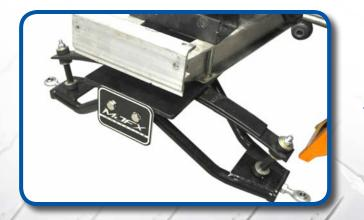
Attach the Main Suspension Assembly using hardware retained from Step 9 and tighten.
