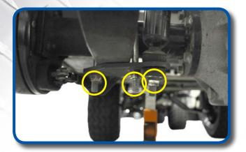
Remove nut from shock and factory U-bolt on driver's side.
