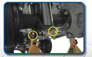
Attach factory lower bracket to U-bolts being sure that the bolt from step 25 fits properly into the hole in the axle.
