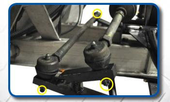
Attach steering linkage to upper portion of spindles on both sides using hardware retained from Step 8 and tighten. Reattach hub and dust cap using hardware retained from Step 4.
