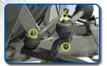
Remove the three castle nuts from steering linkage and retain all hardware.
