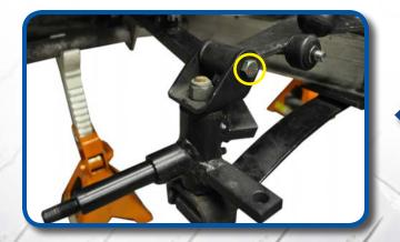
Remove A-Arm bolt from factory spindle on both sides.
