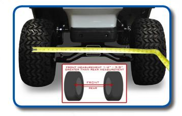
To adjust toe-in/toe-out, loosen nut on both tie rod ends. Adjust using a wrench to desired alignment.
