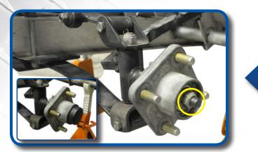
Remove dust cap, then remove nut from spindle. Retain hub and hardware.
