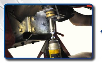
Carefully lower the jack until the bolt threads extend throught the small hole on the new engine mount bracket. Tighten the bolt and hardware using the 15mm socket.
