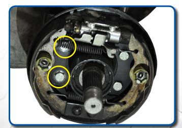
Remove the 2 bolts with a 13mm socket on the brake assembly connected to the brake cable bracket, and remove jam nut on brake cable from brake cable bracket. Discard bracket. Retain hardware.
