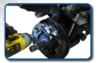
Install the new brake cable bracket in the same location where the original one was removed using the original hardware. Tighten. Reinstall the hub onto the axle using the original castle nut and cotter pin. Tighten.
