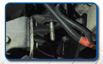
Place the new engine mount bracket where old motor mount was removed. The engine mount tab will face the rear. Install the engine mount bracket using the original hardware. Tighten the hardware. Place the Bolt provided and hardware through the front engine mount hole. Place Madjax plate washer on top of factory motor mount. Place all washers, cap adapters and the compression spring in their original locations in relation to the front engine mount and the new engine mount bracket.
