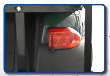
Using a wire snake, pull the tail light connector through the hole in the rear body.Connect the tail lights to the vehicle tail light wiring harness. Determine the desired location of the tail lights. Remove the double sided tape from the back of the tail light and mount to the rear body.
