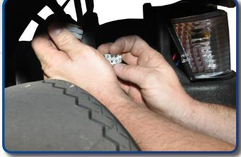
Before removing double sided tape and installing the LED Tail Lights, test fit them in their position on the rear location of the vehicle. Mark the center of the tailight hole using drawing Using a 1-1/2 inch hole saw, drill a hole in the location as shown in drawing 1. Sand to remove sharp edges.
