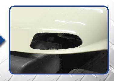
Insert LED headlights and attach to cart using clips located behind the headlight.
