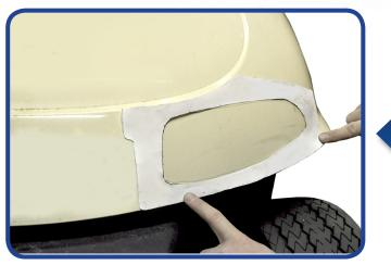
Place headlight template against cart using the body lines for alignment. Draw the inside of the template out with a marking pen.
