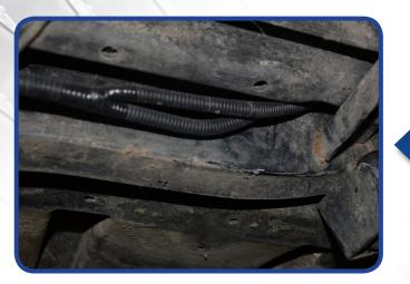
Run wiring harness beside the frame so it doesn't hang. Secure it with wire ties to keep it in place while you are riding.
