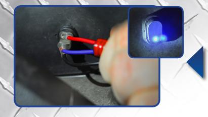
Attach harness to Rocker Switch as shown.
