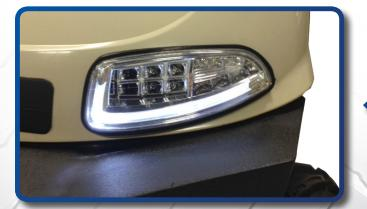
When you turn on the key switch the daytime run lights will now come on. They will stay on when you turn on the headlights and will only turn off when the keyswitch is off. Run wiring harness down the side of the frame of the cart as shown.
