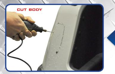
Using the template you drew on the cart, cut out the light area of the body starting at the pilot hole from step 2.
