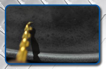
Using a 15/32" drill bit, find a desire location on your golf cart dashboard. Drill gently to ensure nothing is damaged.
