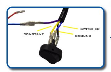
For RXV, DRIVE, FREEDOM TXT, AND TXT LIGHT BAR remove dash to access rocker switch. Yellow and blue wires from indicator harness go into rocker switch which will operate the hazard lights only. The purple wire from the indicator harness connects to the blue wire on main harness. (red is not used)
