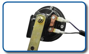
Attach horn to purple and black female spade connectors and secure horn under front cowl.
