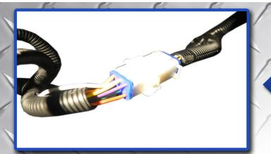
Connect 9 pin connector from signal indicator to 9 pin connector on harness from light kit.
