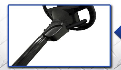
Attach column cover to steering column, secure harness in column cover void.
