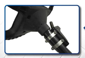
Mount indicator assembly using clamps provided and tighten. Run indicator harness along steering column and insert harness through dash.
