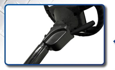
Attach column cover to steering column, secure harness in column cover void.
