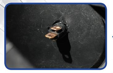
Feed threaded end of switch through the dash where the hole was drilled. Attach the nut to secure the harness.
