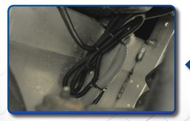
Secure remaining harness under cowl using provided ties.
