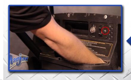
Remove cup holder.Feed threaded end of switch through the dash where the hole was drilled. Retain hardware\* Mount indicator assembly using clamps provided and tighten. Run indicator harness along steering column and insert harness through dash.
