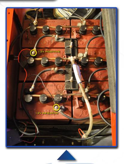
IMPORTANT: This light kit is designed for 12V power. A Madjax 16/12 voltage reducer will be needed if no 12v power available.
