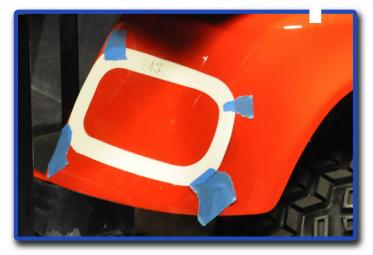
Place tail light template against cart. Using a writing utensil, draw the template onto the cart. Repeat on opposite side and be sure to reverse (flip over) template.
