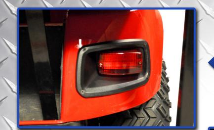
Attach tail light to harness, then insert tail light and attach tail light to cart using provided hardware. Connect red connector on harness to passenger side lights and white connector to driver's side lights.
