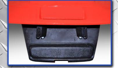
Install mounting brackets with mounting holes facing out using hardware retained from step 1.
