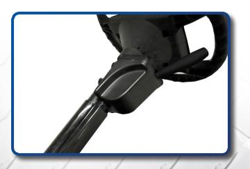
Attach column cover to steering column, secure harness in column cover void.
