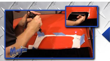
Cut out the shape of the headlight. \*Use the cutting tool to remove the excess trim. Keep your template for the other side.
