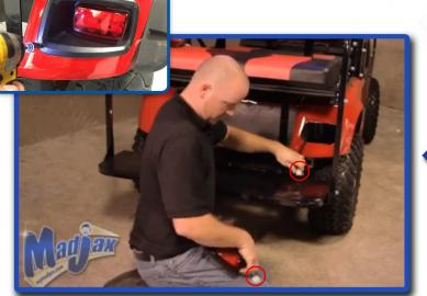
Attach rear tail light wire harness. Then place tail light into the rear of the vehicle. Insert four screws into tail light using supplied hardware. Secure wire with ties. \*Repeat process on other side.
