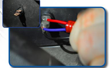
Attach harness to rocker switch as shown.
