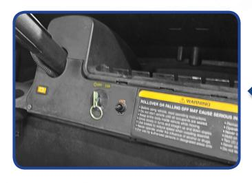
Drill hole in dash slightly larger than switch and install switch. Route black wire to a good ground (12 volt)\* and the red wire to a 12 volt \* source.
