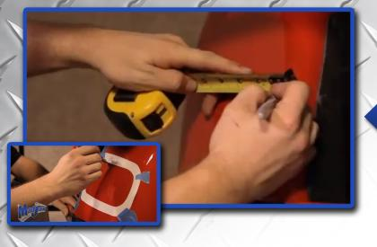
Using the measurements provided on your tail light template, measure and mark your template. Use a marking pen to trace the inside line. \*Flip template over to use on other side.
