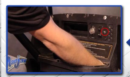
Remove cup holder. Feed threaded end of switch through the dash where the hole was drilled. Retain hardware\*
