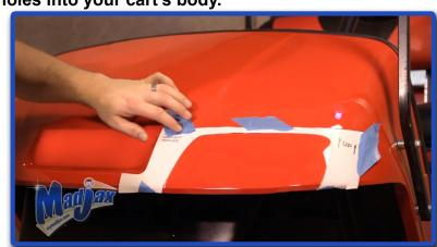
Drill pilot hole on the inside of the template line.
