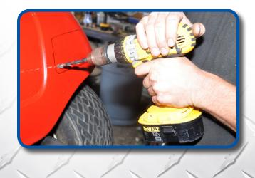
Drill pilot holes on the INSIDE of the marks as shown.
