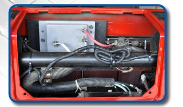
Use the supplied zip ties to fasten wiring harness to vehicle . MadJax recommends fastening the wiring harness to frame members in the front of the vehicle in order to prevent the harness from making contact, rubbing, or being pinched by moving parts, such as the suspension. Use two zip ties to tie the wiring harness to the frame at the back of the motor compartment as shown. Replace motor cover.
