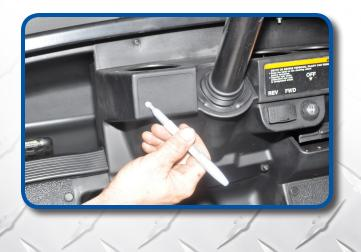
Locate a place on the dashboard to mount the switch. We recommend using the location shown as it does not interfere with the cup holder when reinstalled and also allows you to easily route the wiring harness.
