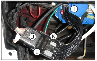
NOTE: The Module should be oriented and secured with Zip Ties so that water and debris does not accumulate in the Connectors.
