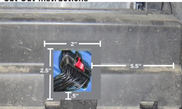
If the Precedent has a six 8V Battery layout, the plastic on Controller/Wiring Cover will need to be cut out to allow the 20 pin Connector on the Vehicle Module Harness to fit properly. Caution: Remove the Vehicle Module Harness before cutting in to the plastic Cover.
