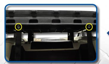
Using hardware Pack 3, mount bagwell bracket to frame as shown.
