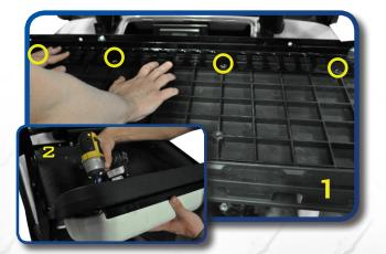
1. Place HD bracket on flip seat as shown. Align bracket holes to the flip seat mounting holes.
