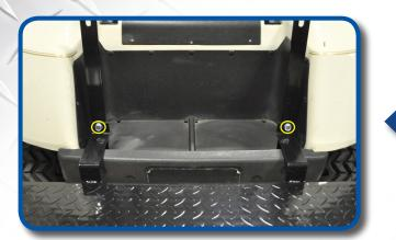
Attach footrest as shown using remaining hardware from Pack 3.
