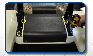
Install main brackets using hardware from Pack 1. Position the brackets as shown. Tighten hardware. Mount the Bagwell brackets to the **OUTER** holes using hardware Pack 2.
