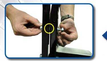
Using the hardware from Pack 5, attach the seat back support bracket and the armrest in two locations. Mount provided rubber spacer inbetween the armrest and seat back support bracket. Repeat process on the other side.
