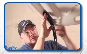
After rear struts are attached, remove brace. Insert rear struts into canopy channel. Using hardware retained from Step 1, attach rear struts to the canopy. Using remaining hardware from Pack 5. Install the foot rest brackets. Bracket goes behind armrest and under footrest. Repeat process on other side and then tighten hardware.
