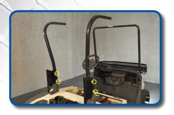
Attach rear struts using retained hardware from Step 1. Tighten hardware.
