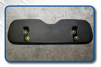
Attach seat back brackets to seat back using hardware from Pack 5.
