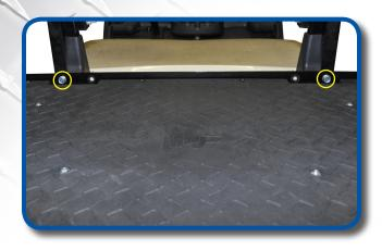
Attach seat frame to brackets using remaining hardware from Pack 2. Tighten hardware.
