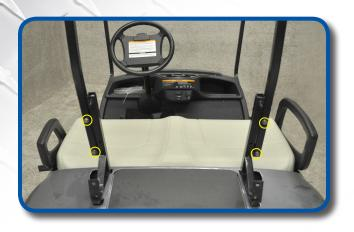
Attach rear struts to front brackets using hardware retained from Step 3.
