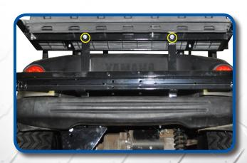
Attach seat frame to bagwell brackets using hardware from Pack 1.
