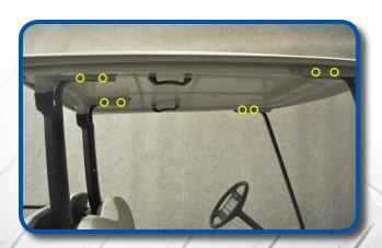
Using hardware retained from Step 1, re attach canopy as shown.
