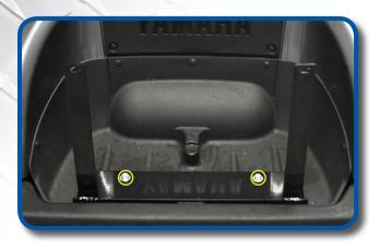
Attach bagwell bracket using hardware from Pack 2.
