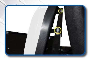
Attach seat back to seat back support using hardware from Pack 5. Tighten all hardware.
