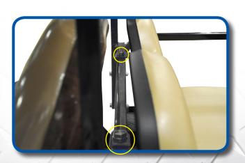
Attach seat back to seat back support using hardware from Pack 4. Tighten all hardware.
