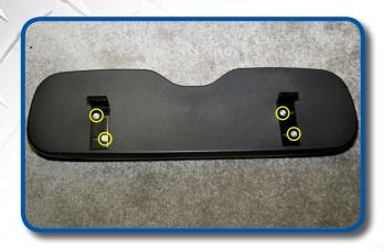
Attach lean back brackets to seat back using hardware form Pack 5.
