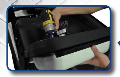
Make sure the thickest part of the seat bottom points towards the footrest. Center seat bottom from left to right on flip frame. Press cushion firmly against HD bracket and seat frame. Using provided hardware tighten the seat bottom to seat frame as shown.
