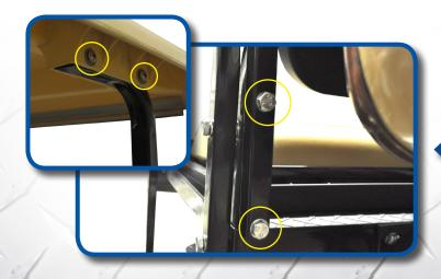
Attach new rear struts to seat back support using hardware from Pack 4. Attach canopy hardware retained from step 1.
