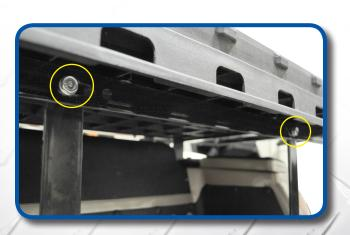
Attach seat frame to bagwell brackets using hardware Pack 2.
