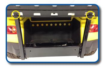
Attach seat frame to bagwell bracket supports using two small head 10mm x 50mm bolts from pack 2. Once both bolts are in place, tighten.
