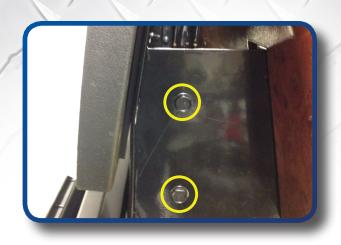
Attach factory top to front struts and new rear struts using hardware retained from Step 1.
