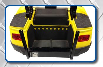
Place bagwell bracket over bumper as shown. This will be mounted later and only used as a support to install the frame for now.
