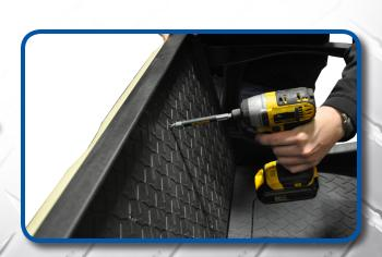
Attach new struts to main brackets using four 10mm x 45mm bolts from Pack #6 as shown.
