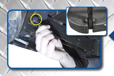
Using quick release clips from hardware pack 6 Secure footplate to bagwell bracket and grab bar as shown.
