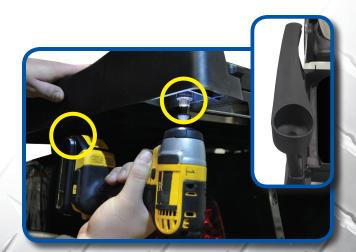
Using appropriate hole for your cart attach lean back brackets to main seat bracket using hardware from pack 4.
