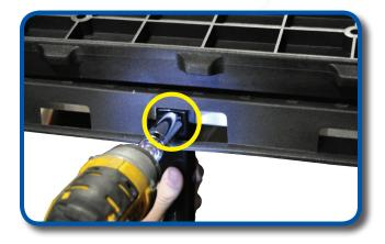
Attach bagwell bracket to to polyboard seat frame as shown using hardware from pack 2. Repeat process on other side.
