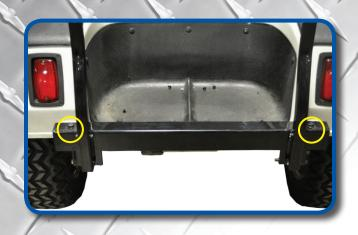
Attach bagwell bracket to frame as shown using hardware from pack 2 and tighten.
