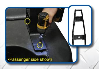
Attach main brackets to cart using hardware from Pack 1 at same location as step 5.
