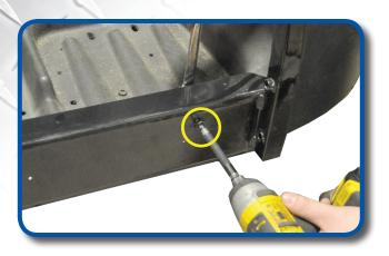
Using a #3 phillips head bit, attach bagwell bracket to cart using hardware from Pack 3.
