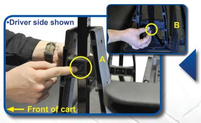
Place rear struts through main seat brackets as shown, use provided hardware remaining from Pack 1. Repeat process on other side.
