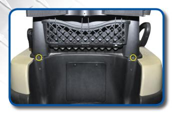
Remove hardware from base of basket. Two bolts are located in the rear and two bolts located in the front.
