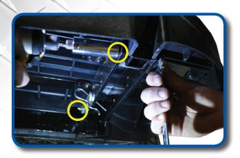
Attach grab bar to footrest as shown using 10mm hardware from pack 7. Repeat process on other side.
