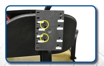
Using the appropriate labeled hole for your cart attach lean back bracket to main seat bracket using hardware from pack 4.
