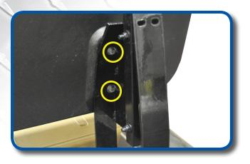
Attach factory lean back cushions using hardware retained from step 1.
