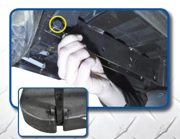
Secure footrest as shown using quick release clips from hardware pack 6.
