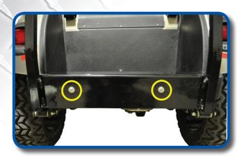
Attach bagwell bracket to rear of cart as shown using hardware from pack 2.
