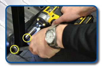
Attach footrest to bagwell bracket using 10mm hardware from pack 6. Repeat process on other side and tighten.
