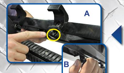
A) Loosen threaded knob on bottom of rail attachment and slide Golf bag holder onto rail.B) Tighten rail attachments to rail using threaded knobs in desired location.
