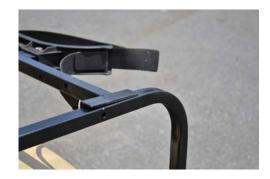
5. Line up Golf Bag Attachment Bar assembly with hole and fasten to armrest with threaded knobs.
