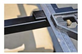
4. Strike a vertical line on the armrest to mark drill location. Drill through armrest.
