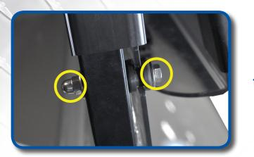
Using provided hardware, mount the windshield to the front struts.
