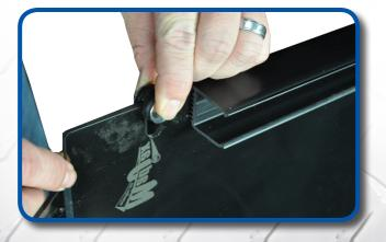
Using rubber grommet provided, insert hardware. Repeat this process on the other side.
