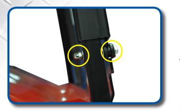
Tighten windshield. Be careful not to overtighten and break windshield.
